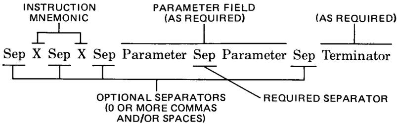
**NOTE:** The syntax implemented on the 7470 is extremely flexible and differs from that used on other Hewlett-Packard plotters such as the HP 9872. Therefore, any software written for the 7470 which takes advantage of its less rigorous syntax will not be able to drive most other HP plotters. If software is to be used with other HP-GL plotters, the more rigorous syntax of the HP 9872 plotter should be used.
