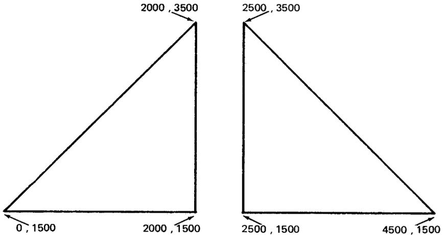
The next strings of HP-GL instructions scale the plotting area into user units 0 to 100 in each axis and again draws two triangles. Use an output statement implemented on your computer to send the strings to the plotter.
