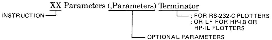
The 9872 syntax does not allow separators between the characters of the mnemonic. One comma must separate parameters. Only ; or LF may be used as the terminator for HP-IB or HP-IL plotters, and only ; may be used as the terminator for RS-232-C plotters. In addition, parameters requiring integer format may not contain a decimal point or decimal fraction. ■
