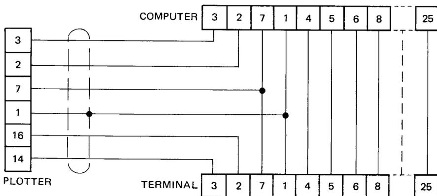
PINS 4, 5, 6, AND 8 THROUGH 25 ARE DIRECTLY CONNECTED BETWEEN THE
