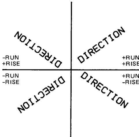
A change in P1 or P2 will affect the direction of lettering. Refer to the section Parameter Interaction in Labeling Commands.
