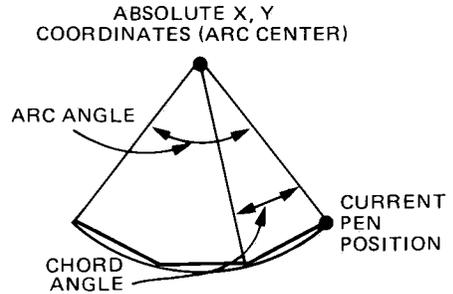
**EXPLANATION** The AA instruction requires that both X- and Y-coordinates be specified (coordinate pair) in integer format. They are interpreted as plotter units if scaling is off or as user units if scaling is on. The X- and Y-coordinates locate the center of the arc and may be located on or off the plotting surface. The current pen position is the starting point of the arc.
