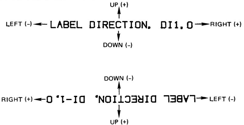
The pen's position (raised or lowered) does not change when a CP command is executed. The parameters must be  $\geq -128$  and  $< +128$ . However, since there are approximately 90 character-space-field widths and 40 character-space-field heights on the plotting surface, assuming default sizing, the effective parameter range that will keep the labels on the medium is considerably less, depending on the pen position at the given time.
