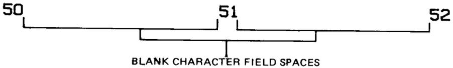
The following example illustrates the closer spacing achieved in BASIC when semicolons separate variables in labeling commands. The semicolons between the variables cause suppression of blank spaces. The space between the printed integers varies with different computers, but normally includes the sign space.
