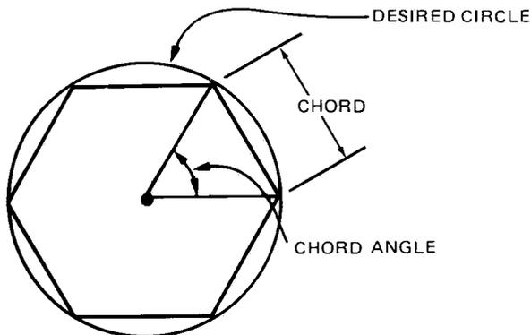
The most useful chord angle values range from 0 to 180; where 0 produces the smoothest circle and larger numbers progressively reduce the number of chords used. Values from 180 to 360 work just the opposite; i.e., larger numbers progressively increase the number of chords used and 360 produces the smoothest circle. This pattern follows modulo 360 through the permitted range of -32 768 to -32 767. Specifying out-of-range parameters sets error 3 and the command is ignored.
