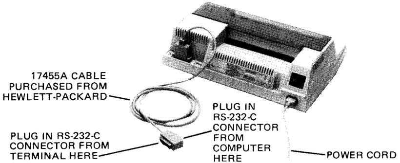
Plotter Interconnection with a Terminal and Remote Facility
