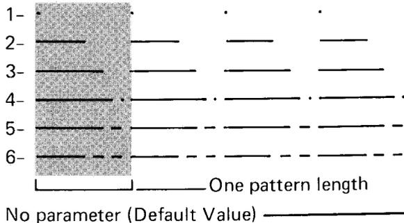
The shaded portion of each of the line patterns above is one complete segment of the pattern.
